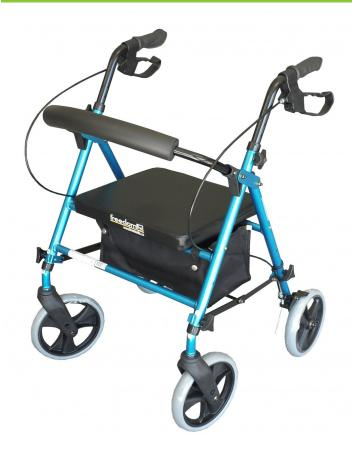
An aluminium, folding, four wheel walking frame. It has a padded seat and a removable vinyl storage bag located under the seat. Features include a removable rounded padded backrest, height adjustable contoured hand grips and cable hand brakes. Seat height is also adjustable. Two options are available: 6" and 8" castors.
